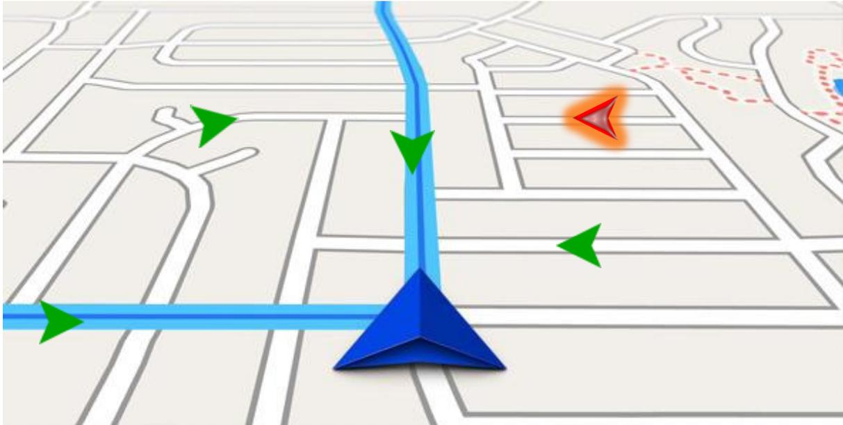
In the figure above, it can be seen a prototype navigation system map with the *green* arrows which indicates the other moving vehicles in the near area, and the *red* arrow which indicates the request-for-aid alarm situation of a car. The *blue* arrow depicts the personal vehicle location and direction.
