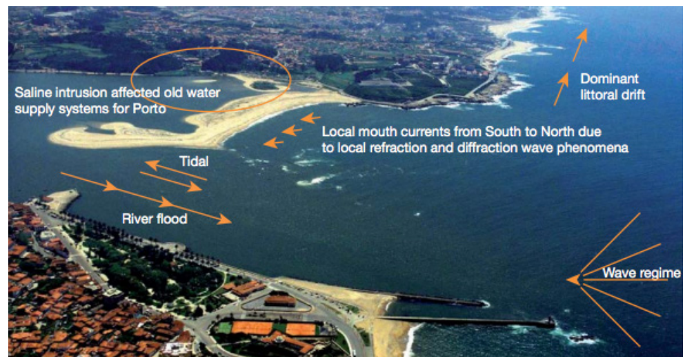
Figure 1: Hydrological and sediment processes at the mouth of the Douro (SedNet, F. Veloso Gomes, 2006)
